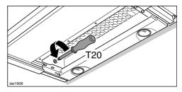
■ Note for dismantling the rangehood: Undoing the screws on the left and right inside the housing releases the spring mounts, allowing the appliance to be removed from the unit.
