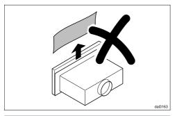
To avoid scratching the deflector plate, do not remove the protective film between the deflector plate and the casing until the rangehood has been placed in the housing unit.
