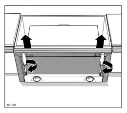
Use a screwdriver to align the deflector plate correctly.
