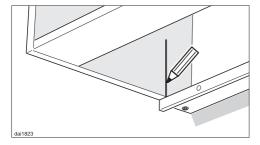
Draw a vertical line up both inside walls of the housing from the front of the spacer strip.
