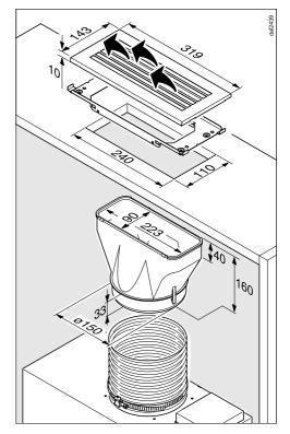
■ Fit the conversion kit as described in the installation instructions supplied with the kit. Make sure that the slats in the exhaust grille point towards the centre of the room and not towards a wall or the ceiling.
