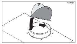
If required, install the non-return flap. Check that the flap opens easily and closes by itself.
