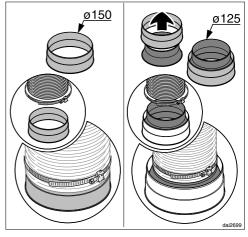
■ Attach the exhaust ducting, e.g. flexible hose, to the exhaust collar using a hose clip (available as an optional accessory). When using Ø 125 mm ducting, fit the reducing collar supplied into the exhaust socket (see "Connection for air extraction").
