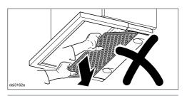
When removing the grease filter do not tilt it downwards at an angle. This can damage the retaining pins.
