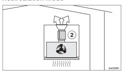
The silencer needs to be positioned between the exhaust connection and the exhaust grille ②. Ensure there is adequate space for fitting it.
