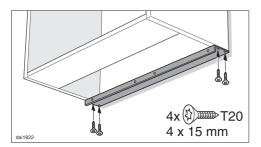
Secure the spacer strip underneath the housing unit sides, flush with the rear wall.
